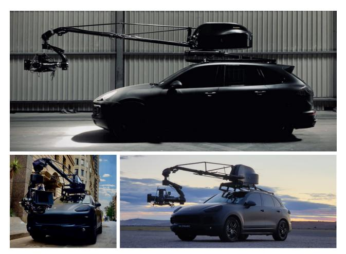
The U-Crane Dynamic is a new generation of our gyrostabilized robotic camera crane systems. It is a remotely operated gyrostabilized minicrane technology that was designed for use on small camera cars, electric carts, process trailers or other small tracking vehicles to be able perform on narrow roads, small sized sets, tunnels, parking garages, bridges.
