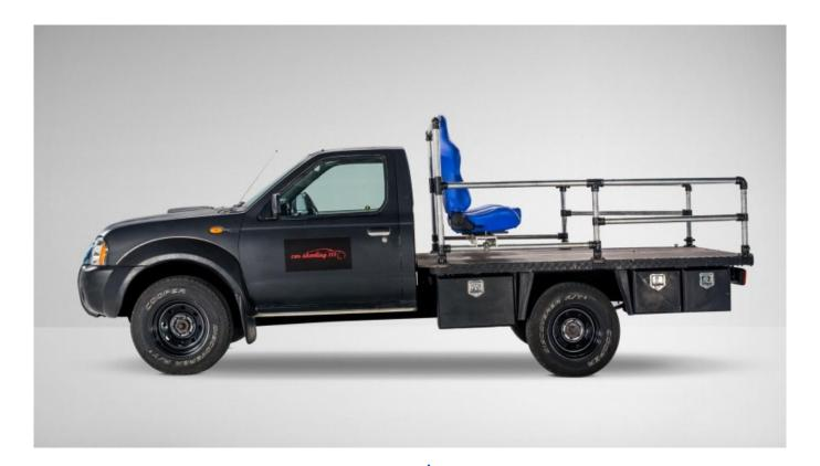
This vehicle is definitely ideal for Car shoots where a small camera car is required. Full equipped for easy grip, tubular structure with 48 mm aluminum, platforms and various adapters.
