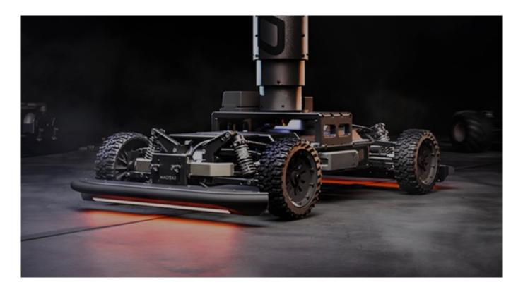
MagTrax enhances the existing Sports drive-ends enabling customers to follow a magnetic strip laid on a surface, underneath a carpet or embedded within a set. The magnetic strip can be arranged in various creative ways beyond what you can do with a regular track.
