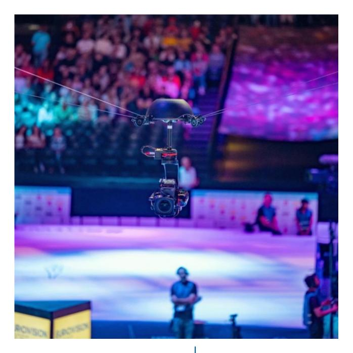
The Eagle Eye opens up a whole new world of camera movement possibilities. The system offers a 3-dimensional (XYZ), a 2-dimensional (V rig) and a 1-dimensional option and can cover a field of up to 250 metres by 250 metres. The camera system is designed to be used at various events such as sports games, concerts, television productions and much more.
