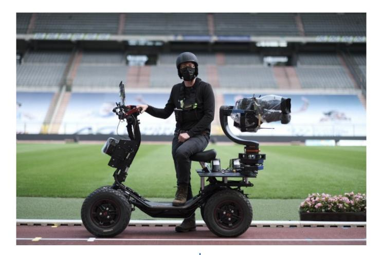
As an electric vehicle, the EZ Raider is almost totally silent. The vehicle is steered via handlebars like a jetski. The electric ATV EZ Raider can be operated over inhospitable terrains, thanks to its unique, field proven characteristics:
