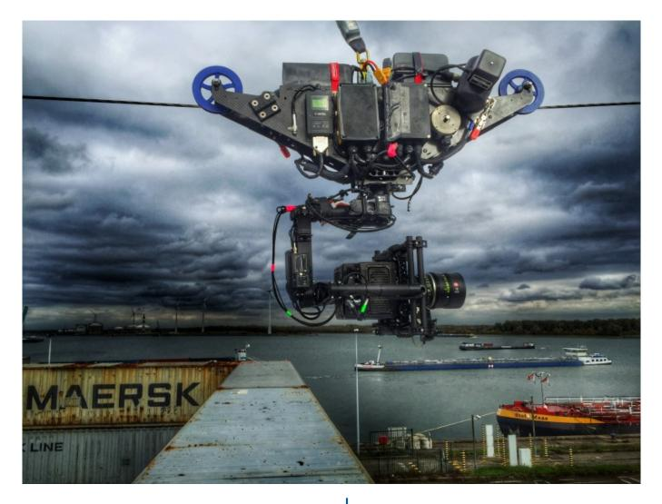
The Flyline is a cablecam system. And this by using two ropes, 1 to ride on and 1 as the safety. The Flyline does not require heavy winches. The Flyline makes use of a DC motor on the trolley along the cable. The power is provided by on-board lithium-polymer batteries. It is possible to reach speeds up to 45 mph (65kph). The maximum rope length is 470m at the moment.
