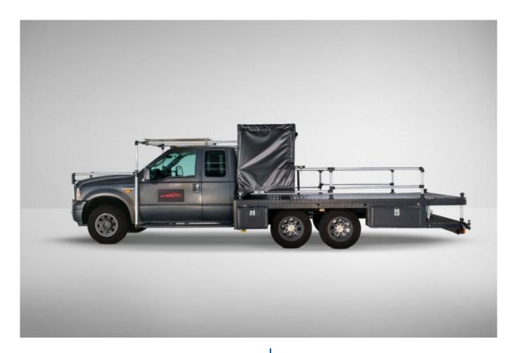
Tracking vehicle with large load capacity and higher drag. Prepared with 48mm tubular structure. There is also the option to put both platforms front and behind.
