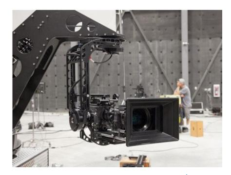
Our precise, robust and light weight 2-axis head for highend digital cinematography is ideal for medium sized camera packages, for example ARRI Alexa with a large zoom lens, such as Optimo 12:1 or Panavision 12:1. At the core of the L40 is our highly robust and precise motor drive with zero backlash, providing lag-free operation.
