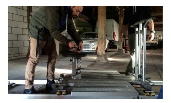
The Sprinter Dolly has a very low weight. It is possible to switch from track-wheels to air tires, within a few seconds without tools.
