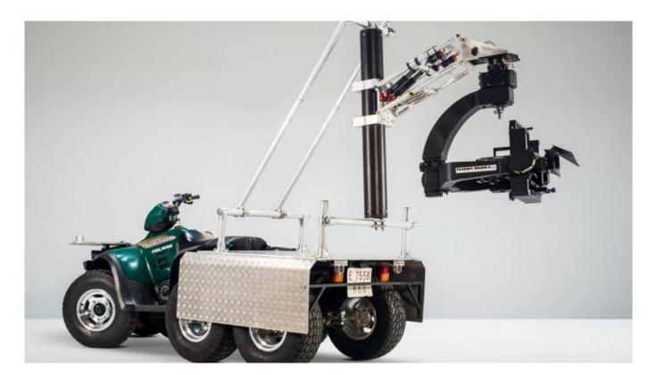
Vehicle designed to capture moving scenes in locations inaccessible or off road (tracks, mountain, beach, etc ...). Both the front and back, is prepared with platform high strength aluminum, to work with 48.3 mm tubular structure. Tambén has wheel arch protectors. We have a caterpillar to work in extreme snow and mud. Very handy for various uses: from working with steadicam operators, as well as to work freehand with various remote heads.
