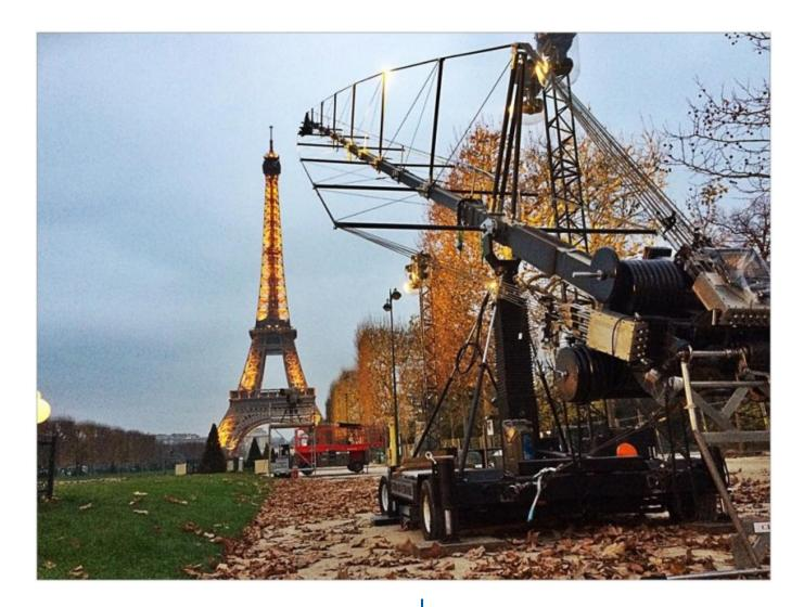
With its maximum length of 100 Feet, The Strada is by far the longest camera crane in the world. This crane allows you to move smoothly and stable from a 10 floors high building to the ground, or to hover -without the use of tracks- over all kinds of surfaces for over 60 meters.
