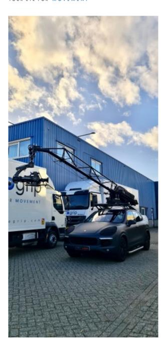
The Topcrane Ghost One is one of the most advanced cranes on the market. This crane is designed and built with performance, efficiency and safety in mind. The Topcrane Ghost One boasts an impressive payload of 36kg / 80lb. It can be used on vehicles with a speed of up to 160 km/h. The topcrane is extremely suitable for all types of weather and terrain conditions.
