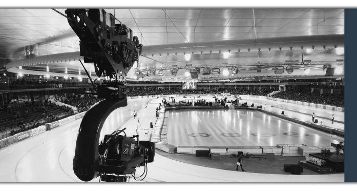
The Flyline is a cablecam system. And this by using two ropes, 1 to ride on and 1 as the safety. The Flyline does not require heavy winches. The Flyline makes use of a DC motor on the trolley along the cable. The power is provided by on-board lithium-polymer batteries. It is possible to reach speeds up to 45 mph (65kph). The maximum rope length is 470m at the moment.
