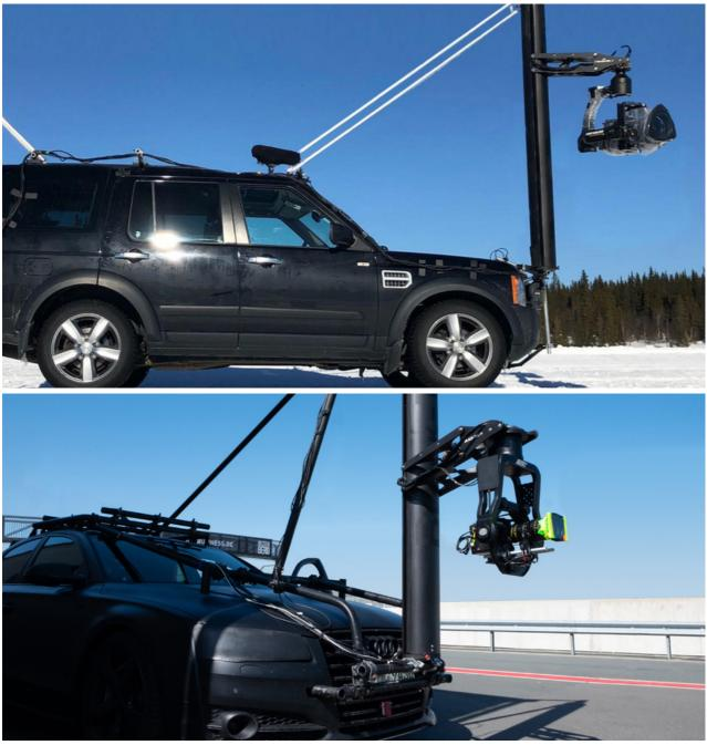
The Tower 24 is a vertical Lifter for Remoteheads and can be mounted on camera cars and or even used stationary. The Tower can be used in conjunction with our Flighthead Mini V4 and V5 and controlled by the camera operator via joystick or foot pedal. The Tower is available to rent separately with a driver and technician as well as a full package which includes the Porsche Cayenne and equipment as listed below.
