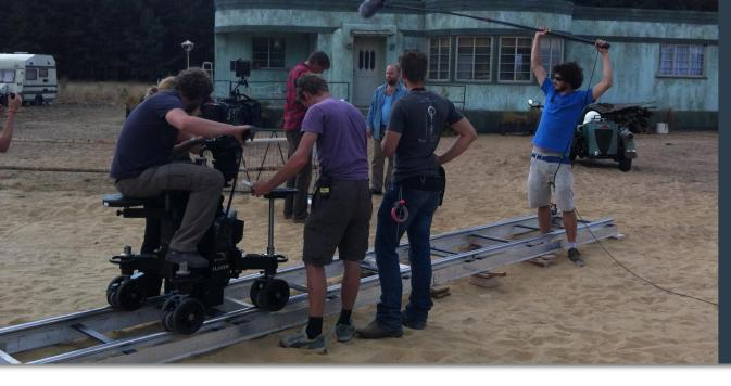
The Panther Classic is the basic Panther model. It has a lot to offer. With its computer-controlled central column and the retractable wheel-arms it can be easily adapted to make the most extreme camera angles. Together with the Panther Classic accessories the possibilities are even greater.
