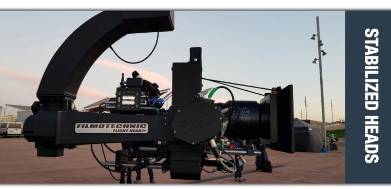
The Flight Head 6 is the regular design of Gyro Stabilised Flight Head from Filmotechnic. But we have the Flight Head 6s. It is a unique head and the only head like this in the world. It has slip rings on all axes. Also on the roll axis so you can keep rolling unlimited 360°!
