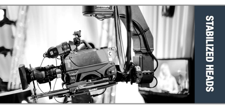
This new 3-axis Flighthead is based on the same technology as the legendary Flighthead 5. This head is designed for the 2014 Winter Olympics in Sochi, and is specially designed for the television market and is ideal for use on telescopic cranes, remote dollies, tracking dollies
